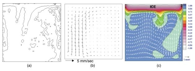
Fig. 15. Typical instabilities measured during the onset of convection: temperature (a) and velocity (b) fields at the centre plane of the cube shaped cavity;  $T_h = 21^{\circ}C$ ,  $T_c = 15^{\circ}C$ ,  $Ra = 2.7 \times 10^{6}$ , Pr = 8; (c) – numerical simulations (h – hot wall, c – cool wall).
