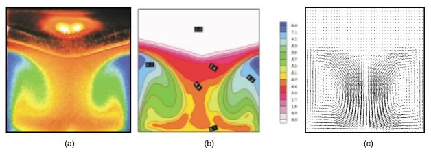
Fig. 16. Freezing of water under cold surface in lid cooled cavity. Recorded image of TLC tracers (a), evaluated temperature (b) and velocity (c) fields. Time step -3600 s after cooling starts; Isothermal lid temperature  $T_c = -10^{\circ}$ C, external temperature  $T_c = 20^{\circ}$ C.
