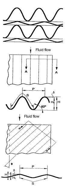
Fig. 7. Working section – general view of corrugated-undulated heat transfer element.
