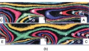
Fig. 8. True-colour images from liquid crystal thermography for an endwall surface with in-line square ribs (left) (a); pattern of ten Nusselt number Nu reconstructed by false colour images of the heat transfer surface for Re = 20000 (No. 0: Nu = 79; 9: 99; 8: 113; 7: 123; 6: 136; 5: 147; 4: 160; 3: 175; 2: 185; 1: 209) (b).
