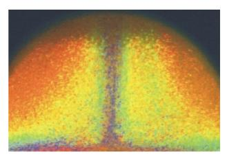
Fig. 13. TLCs visualisation of a thermal aloft generated over locally heated bottom wall of a water basin.
