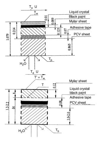
Fig. 3. Liquid crystal package (front print and waterproof).
