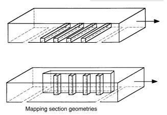
Fig. 6. Mapping section geometries with square roughness elements and rib-roughened channel.
