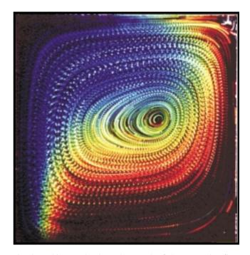
Fig. 4. Multiexposed colour photograph of the convective flow seeded with liquid crystal tracers. Tracers change colour from blue to red following the clock-wise flow circulation from the hot wall (left side) to the cold wall (right side).
