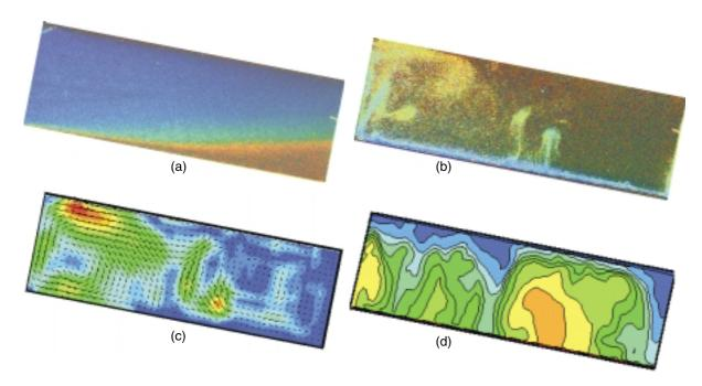
Fig. 14. Convection observed for water in the tilted channel with 11°C temperature difference between top and bottom wall. TLCs visualisation of temperature field for stable thermal stratification (a), visualisation of temperature field with convective instabilities for negative temperature gradient (b), PIV evaluated velocity field with velocity magnitude contours (c), temperature field in the numerical simulation (d).
