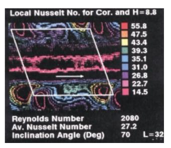
Fig. 9. False colour image of local Nusselt number contours over a central diamond of the undulated plate of corrugated-undulated geometry ( $=70^{\circ}$ , Re =2080, H =8.8 mm, L =32 mm).
