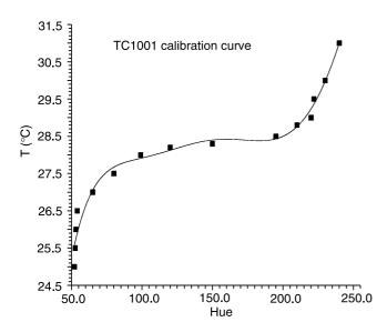
Fig. 5. Temperature vs. hue for TLCs sample used to study natural convection of water. Calibration curve obtained by the 6<sup>th</sup> order polynomial fitted to the experimental points.
