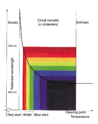
Fig. 1. Typical reflected wavelength (colour) temperature response of a TLC mixture.
