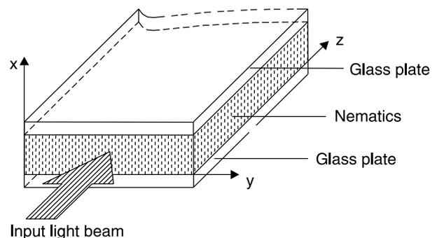
Fig. 1. Schematic of the analysed liquid crystalline waveguides.
