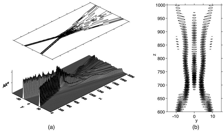
Fig. 4. The same as in Fig. 2 for collisions of solitary waves with higher power (and smaller width).
