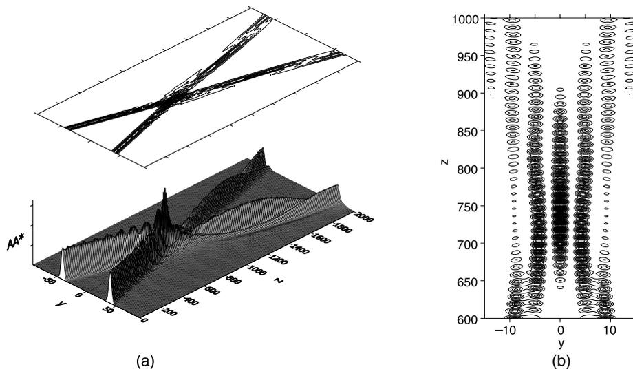
Fig. 2. Collisions of the solitary waves at an angle  $3^\circ$ : the distribution of the light intensity  $|A|^2$  for the TE-field (a) and distribution of the coefficient  $\kappa_1$  in the region of interaction (b). Distances are plotted in micrometers and the light intensity in a dimensionless unit.
