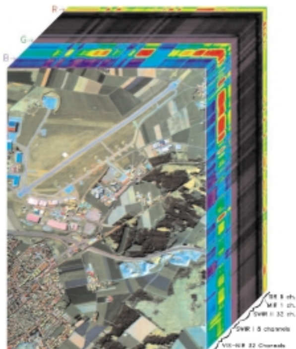
DLR's Research Center at Oberpfaffenhofen Sensor: Digital Airborne Imaging Spectrometer DAIS Flight Altitude: 3000 m, Date: 4 May 1995 Color Composite: R/G/B = 9500/1600/860 nm
