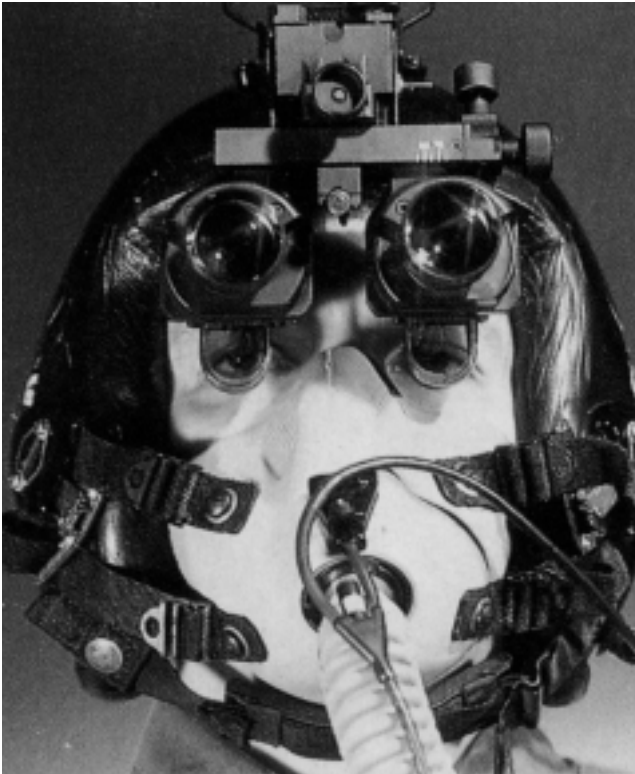
Fig. 13. Marconi Avionics' Cats Eyes incorporate an optical combiner assembly for each eye, allowing the pilot to view the cockpit and the outside world directly with the night imagery superimposed on it. Cats Eyes have a 30° field of view and weight 820 g, including the helmet plate (after Ref. 13).
