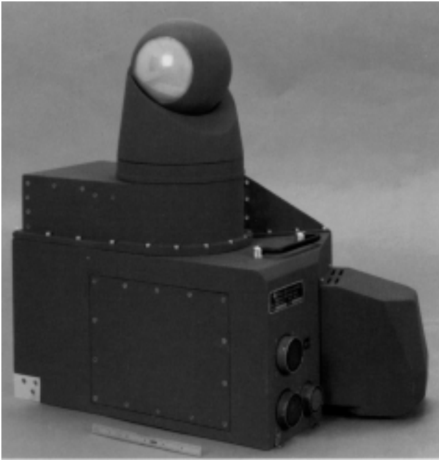
Fig. 22. Falcon Eye, a representative conformal FLIR (after Ref. 18).
