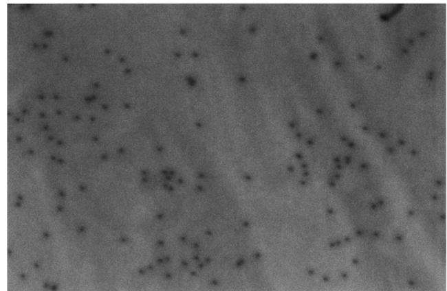
Fig. 4. Cathode luminescence image of  $\text{Al}_{0.22}\text{Ga}_{0.78}\text{N}$  with low density of threading dislocations.
