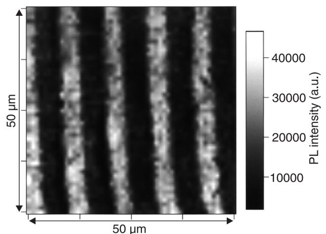
Fig. 2. A micro-photoluminescence (μ-PL) mapping of Ga<sub>N</sub>/AlGa<sub>N</sub> multi-quantum wells grown on the AlGa<sub>N</sub> layer with periodic low density of threading dislocations. The measurement was carried out using He-Cd laser with approximately 1-μm spot at room temperature.
