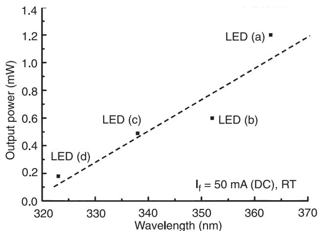
Fig. 6. Output power as a function of peak wavelength at 50-mA (DC) driving current.
