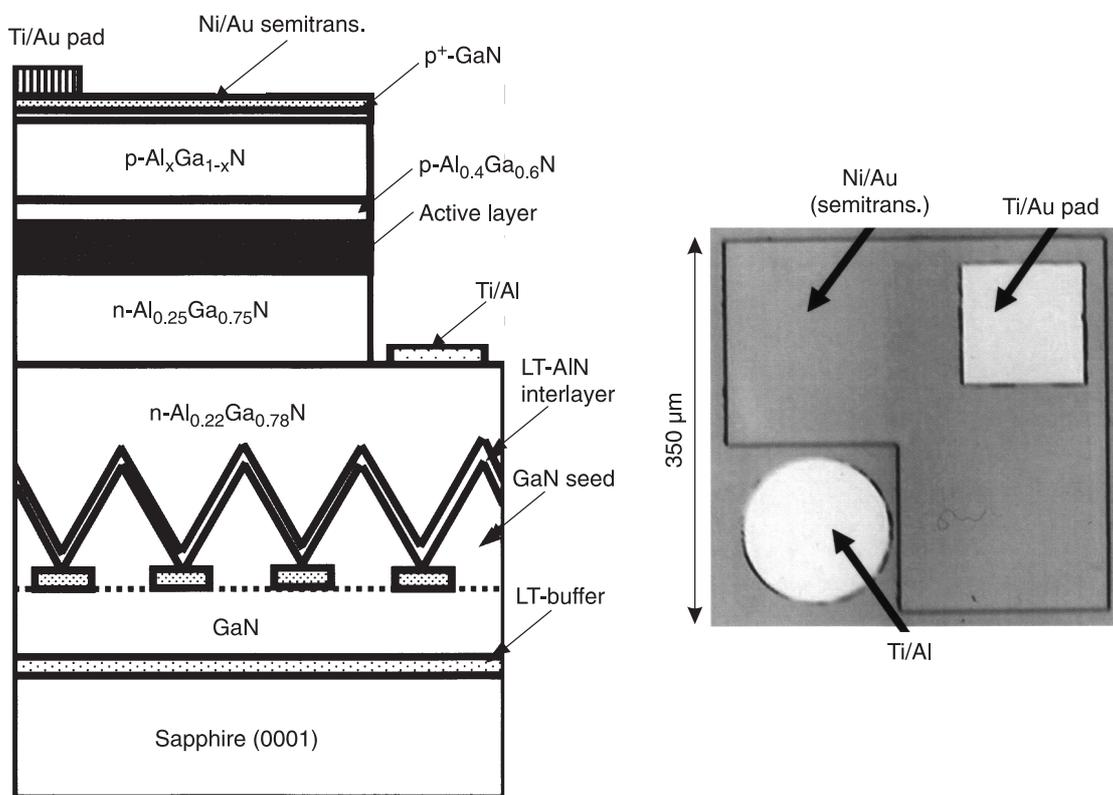
Fig. 5. Schematic UV-LED structure on  $\text{Al}_{0.22}\text{Ga}_{0.78}\text{N}$  base layer with low density of threading dislocations.
