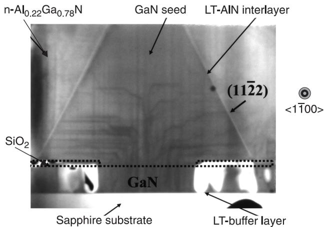
Fig. 3. Transmission electron microscopic image around selectively grown GaN seed crystal with  $(11\bar{2}2)$  facets.
