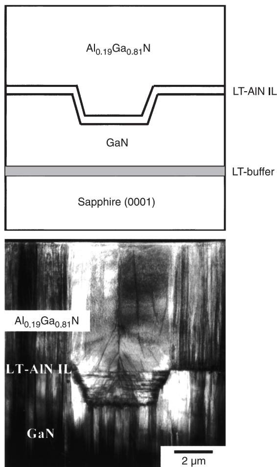
Fig. 1. Schematic drawing and an image of transmission electron microscope of AlGa<sub>N</sub> layer grown on periodically grooved Ga<sub>N</sub> layer through LT-AlN interlayer. The width, depth and spacing of the grooves are 5, 2, and 5 μm, respectively.
