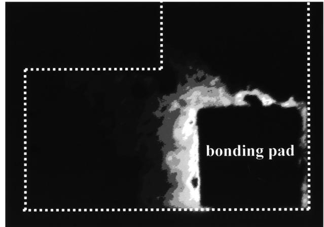
Fig. 7. Output intensity images of LED (c) with emission wavelength of 323-nm. LED is operating at 50 mA (DC).
