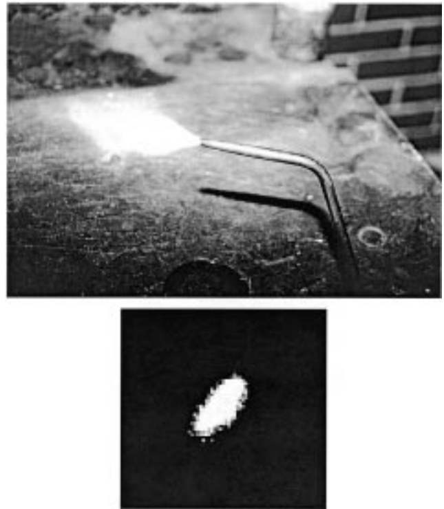
Fig. 7. Visible and UV images obtained for oxy-acetylene torch.
