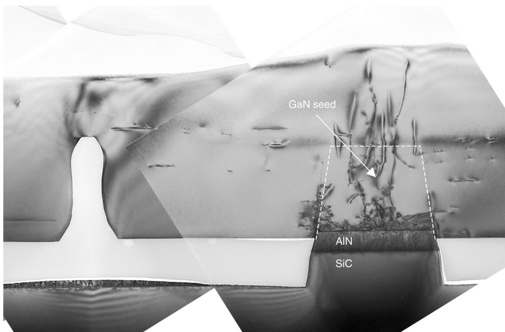
Fig. 2. Composite of cross-sectional TEM micrographs of a PE Al<sub>0.1</sub>Ga<sub>0.9</sub>N film. Note the threading dislocations continue from the GaN stripes into the film.
