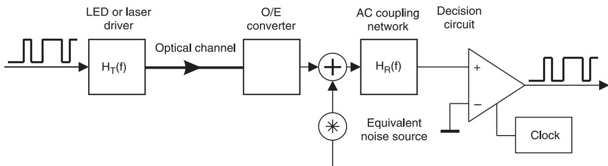
Fig. 1. Block diagram of optical link considered in the paper.
