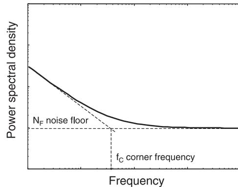
Fig. 2. Power spectral density of equivalent noise source.
