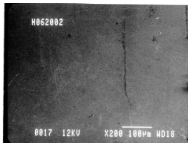
Fig. 11. View of the surface of another GaN wafer, showing a line of defects.
