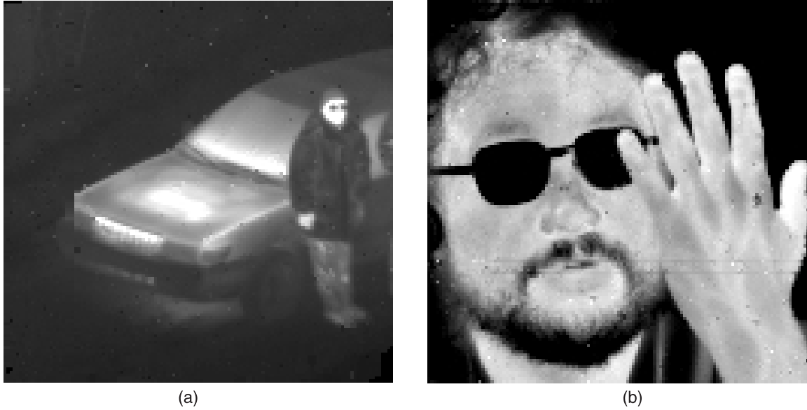
Fig. 12. (a) Thermal image of man and car (FPA, \lambda_c = 6.0 \mu\text{m} ), (b) Thermal image of face and hand with blood veins.
