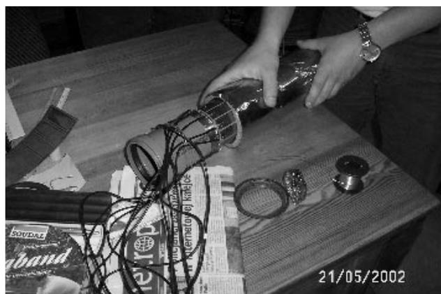
Fig. 3: Twelve electrode sensor.
