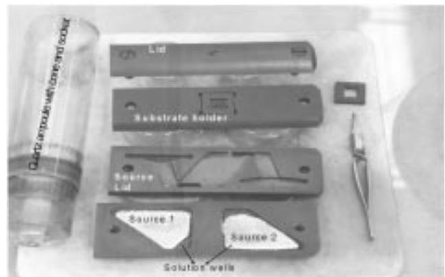
Fig. 4. Graphite boat with two source reservoirs.
