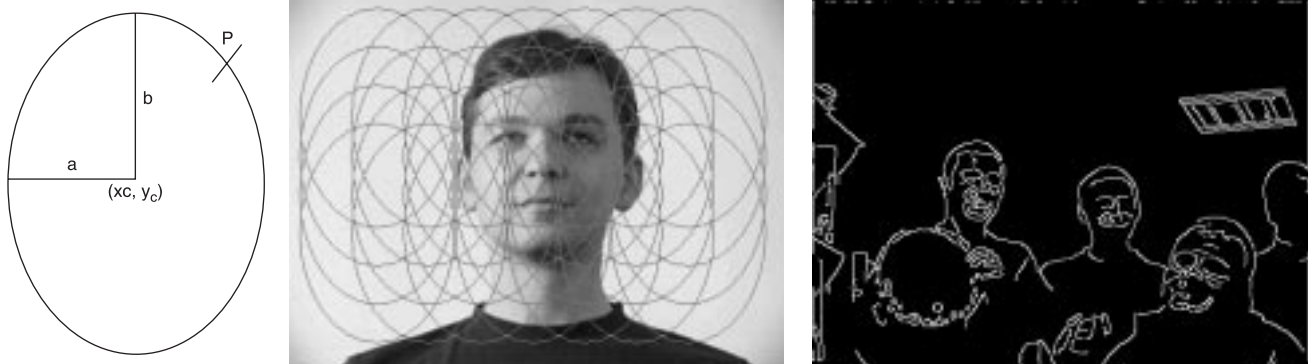
Fig. 2. Hough transform: ellipse parameterisation, sample accumulator, and extracted contours before masking.
