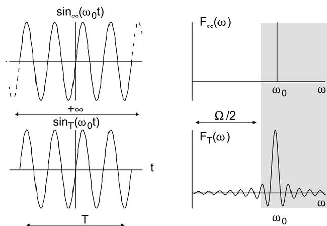
Fig. 1. The  $\omega_0$ -frequency signal (left) of unlimited (top) and  $T$ -limited (bottom) domain, and its spectra (right); dark field denotes frequencies filtered by the transmission channel with cut-off frequency  $\Omega/2$ .
