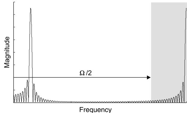
Fig. 6. Spectrum of a signal fragment; dark field denotes the filtered frequencies.
