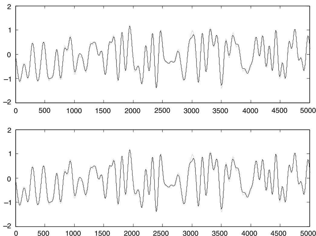
Fig. 9. The signal after transmission through a low-pass channel (top plot) and the restored signal (bottom plot) are compared with the original signal (dotted lines).
