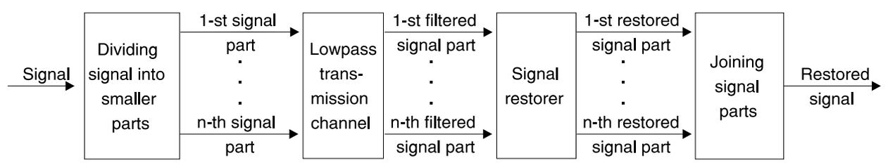
Fig. 4. Diagram of the signal-restoration process by means of signal fragmentation.
