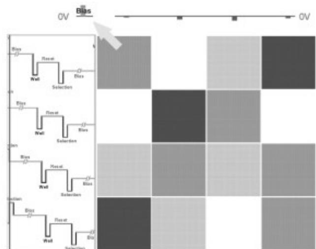
Fig. 3. Multiplexing scheme. Frametime is distributed in as many slots as the number of display rows. Rows are sequentially addressed, each row being delayed one slot from the previous row. The selection pulses extend over the whole row slot to minimize its amplitude.
