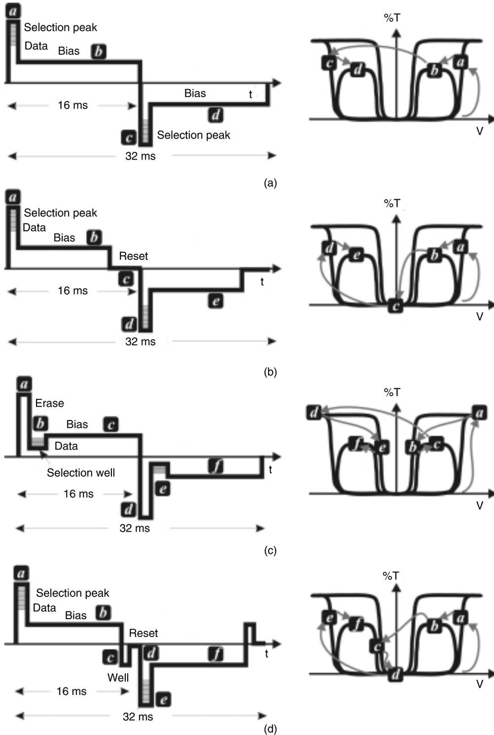
Fig. 2. Classic waveforms used to address multiplexed passive displays. (a) Basic waveform for AFLC driving, (b) same as (a) including a relaxation (reset) step, (c) Waveform based on interframe pixel blanking by saturation, (d) Waveform with forced relaxation to shorten reset time. Data are included onto the selection pulse in (a), (b), and (d). A data well is used in (c).
