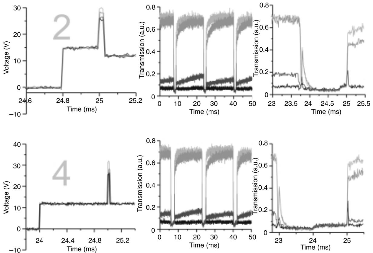
Fig. 6. Grey levels generated by two waveforms with awakening prepulse. A slight transmission increase is observed within the prepulse duration due to pretransitional effect.
