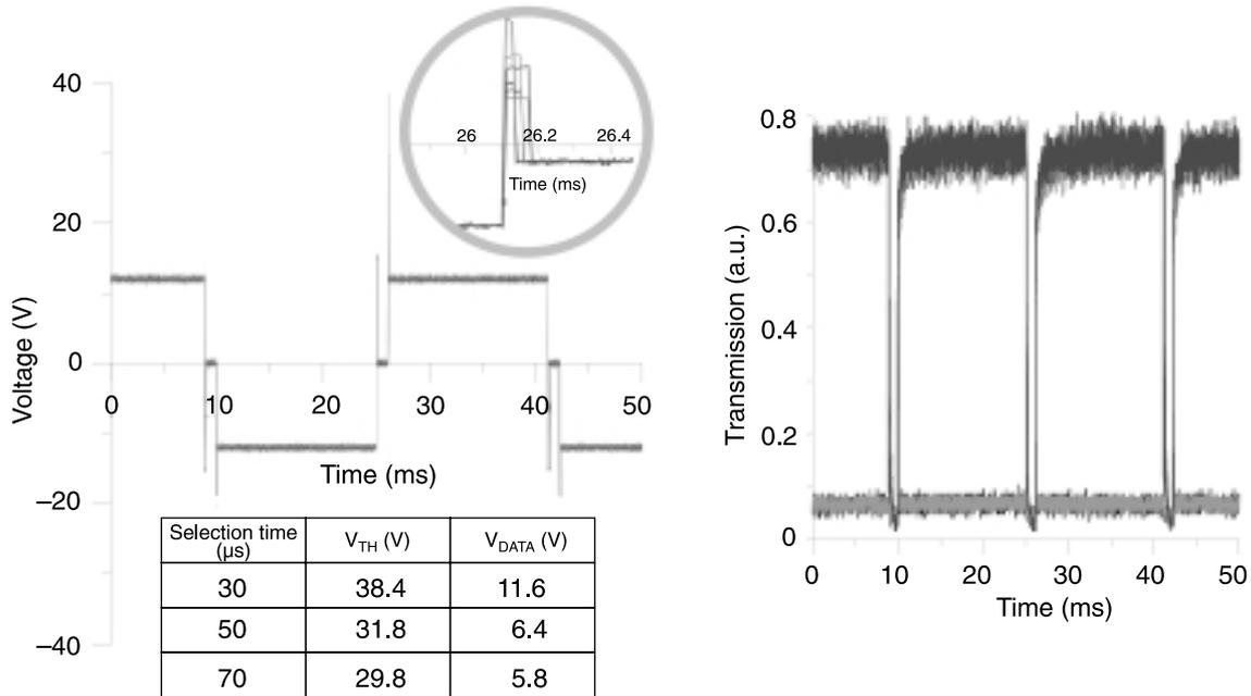
Fig. 4. Variation in threshold voltage and dynamic data range upon reduction of slot time (see inset) corresponding to a video-rate SXGA monochrome display.
