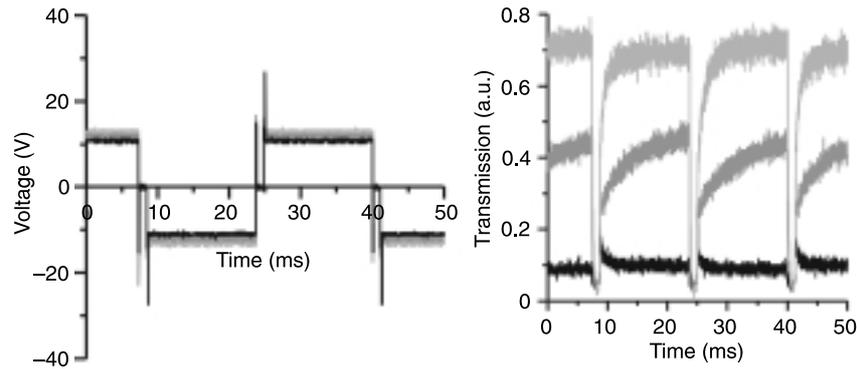
Fig. 7. Three responses obtained for the same intermediate grey level data. Bias levels are modified by the presence of data from other rows. The whole dynamic range has been taken.
