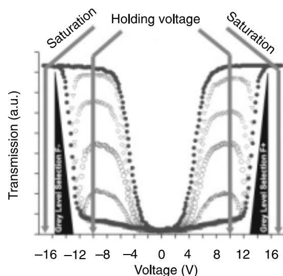
Fig. 1. Low frequency triangular waveform electro-optic AFLC response. Grey level selection is performed on the outer slopes of the hysteresis cycle. When voltage is reduced, different grey levels are shown and held by a constant voltage.
