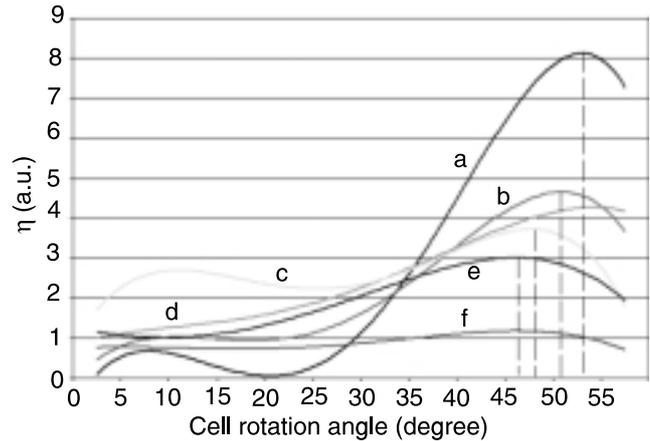
Fig. 3. Dependence of diffraction efficiency and period diffraction grating on cell rotation angle for different LCs parameters: (a) ITO, (b) ITO + orientation layer ( $\Delta n = 0.4$ ), (c) ITO+SiO<sub>2</sub> (100  $\mu\text{m}$ ) + orientation layer, (d) ITO + orientation layer, (e) ITO + orientation layer ( $\Delta n = 0.6$ ), and (f) ITO + SiO<sub>2</sub> (50  $\mu\text{m}$ ) + orientation layer.
