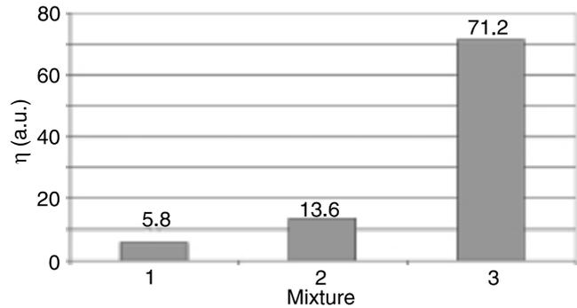
Fig. 7. Diffraction efficiency for LC cells containing mixtures with different optical anisotropy: 1 –  $\Delta n = 0.35$ , 2 –  $\Delta n = 0.4$ , 3 –  $\Delta n = 0.6$ .
