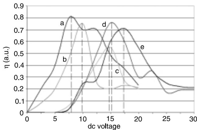
Fig. 2. Dependence of diffraction efficiency on dc voltage value for different orientation layers and LC with  $\Delta n = 0.35$ : (a) ITO, (b) ITO+orientation layer, (c) ITO+PVCN+F, (d) ITO+SiO<sub>2</sub> (50  $\mu\text{m}$ ) + orientation layer, and (e) ITO+SiO<sub>2</sub> (100  $\mu\text{m}$ ) + orientation layer.
