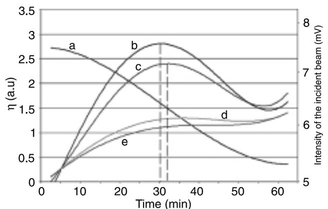
Fig. 4. Dependence of incident writing beam and first order diffraction efficiency as a function of different value DC electric field for LC cell with homeotropic orientation: (a)  $I_0$  intensity, (b) applied voltage polarisation (– +), (c) applied voltage polarisation (+ –), (d) applied voltage polarization (– +), and (e) applied voltage polarization (+ –).
