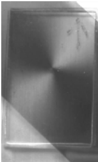
Fig. 2. Light reflection on the filter when corners of the filter are not covered with the polarising sheet.
