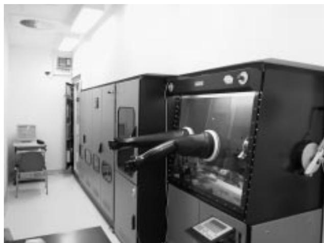
Fig. 1. Aix-200 II–VI system installed at VIGO/WAT MOCVD Laboratory.
