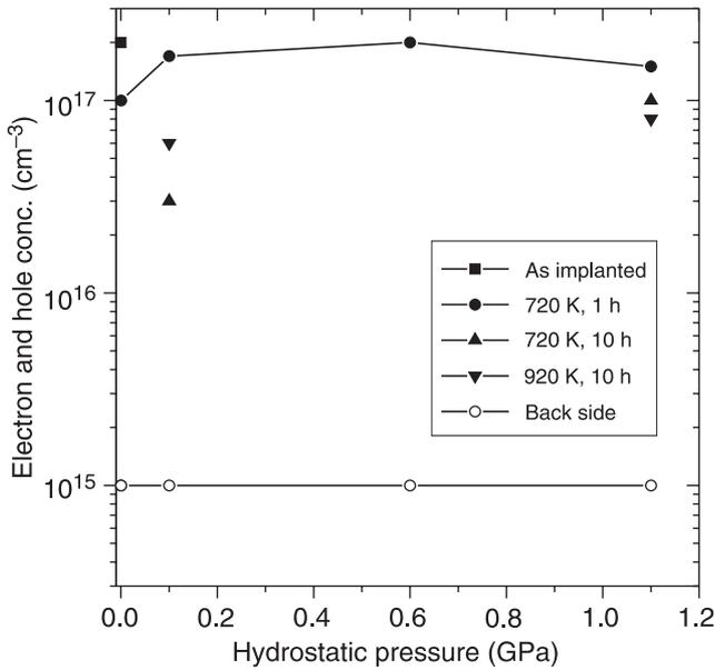
Fig. 5. Carrier concentration dependence on heat treatment under hydrostatic pressure for Si:He,H sample (solid points – electron concentration, open points – hole concentration).
