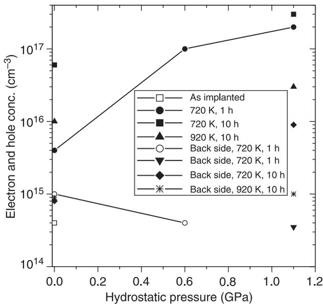
Fig. 6. Carrier concentration dependence on heat treatment under hydrostatic pressure for Si:He,H sample (solid points – electron concentration, open points – hole concentration).
