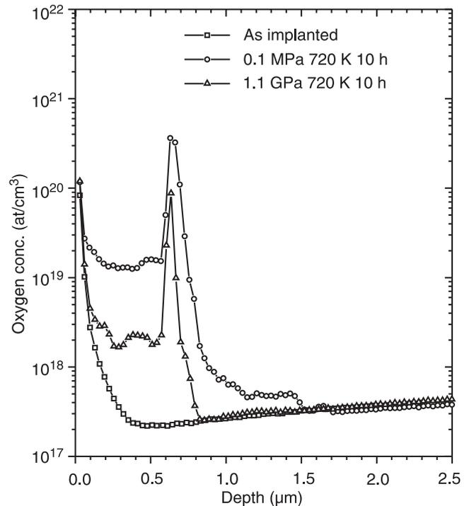
Fig. 4. Oxygen distribution in Si:He,H sample annealed for 10 hours at 720 K.
