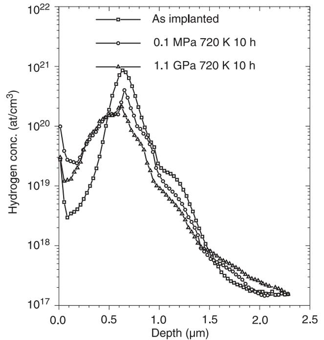
Fig. 3. Hydrogen distribution in Si:He,H sample annealed for 10 hours at 720 K.
