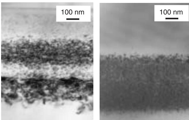
Fig. 2. XTEM images of Si:He,H (left) and Si:H,He (right) annealed for 1 hour at 920 K under pressure of 1.1 GPa.
