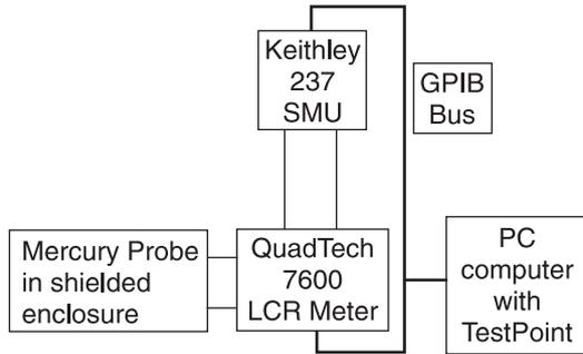
Fig. 1. Block diagram of electrical measurements setup.
