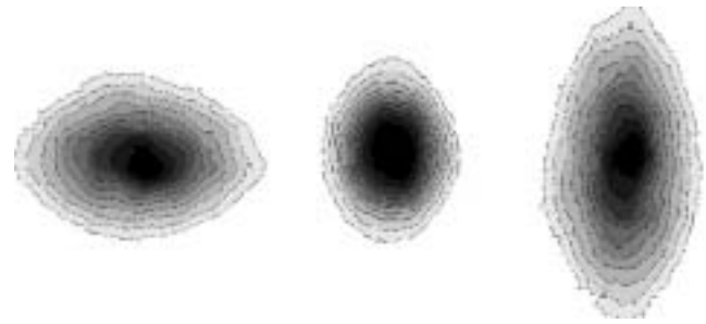
Fig. 7. Thermally induced astigmatic beam of passively Q-switched Nd:YVO 4 laser operating at 1340-nm wavelength, left hand picture – 20 mm before waist, middle picture in the waist, right hand picture 20 mm after the waist, and frame size 1.8 mm.
