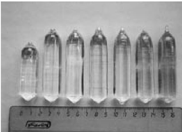
Fig. 1. YAG:Yb single crystals (from left to right 1, 1.5, 2, 3, 5, 7, and 10 at.%; the scale is in cm).
