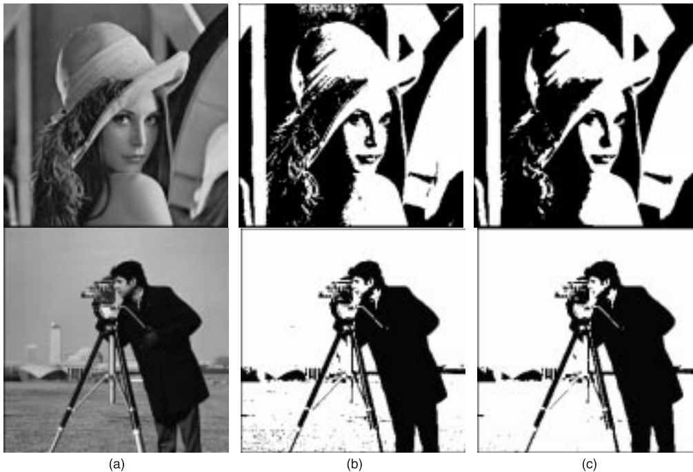
Fig. 4. Comparison of segmentation results on real standard images named Lena and cameraman, (a) the original images, (b) FCM results, and (c) PFCM results.
