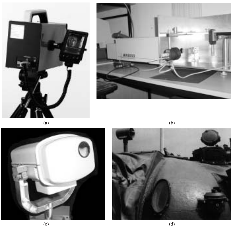
Fig. 12. Infrared systems with Polish HOT photodetectors developed: (a) V-20 thermal imager [54], (b) MIR 8000 FTIR spectrophotometer (Oriel Corp., USA), (c) free space optical communication system (Maxima Corp., USA), and (d) Polish “Obra” tank laser warning systems [56].
