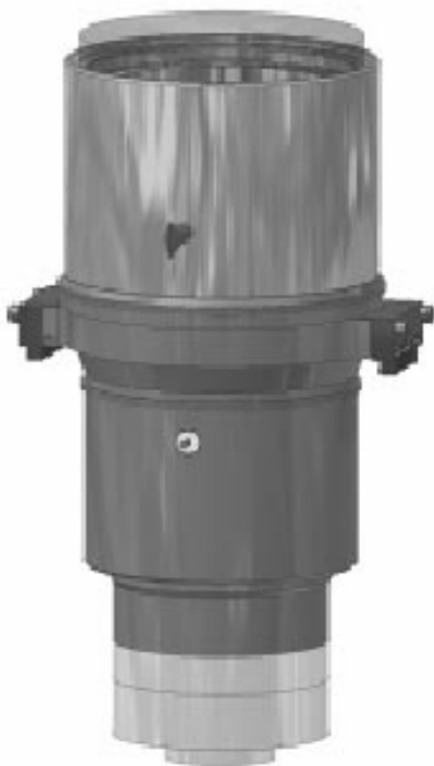
Fig. 19. Dewar design for the 1280×104 MWIR.
