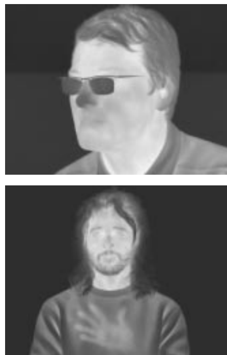
Fig. 18. Images with the Venus-LW camera, focal plane temperature 77 K, simple 2-point NUC.
