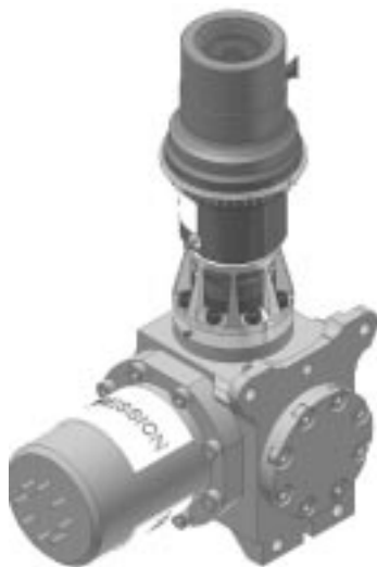
Fig. 10. 320×256 IDDCA with 1/4-W cooler and 30-μm pitch IRFPA.
