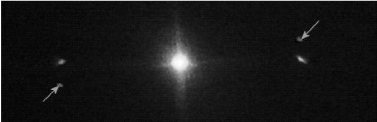
Fig. 4. Observed hologram. Arrows show reconstruction of the stored hologram.
