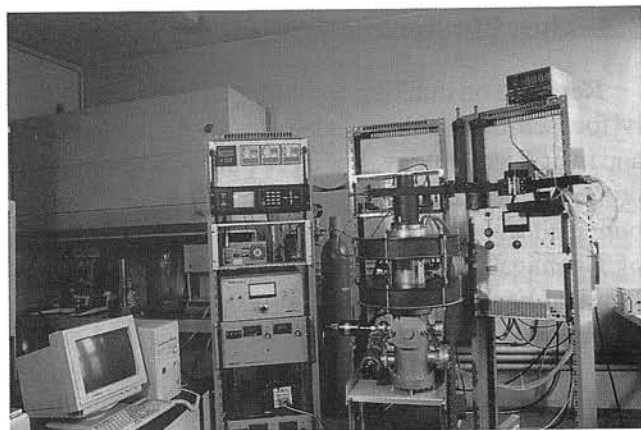
Fig. 4. Electron Cyclotron Resonance Plasma Assisted CVD system.
