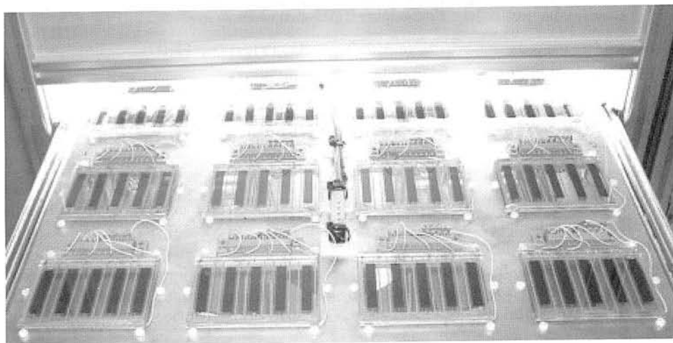
Fig. 6. A series of masterplates placed in a stability test stand.
