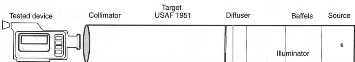
Fig. 8. Optical diagram of a measuring set for testing of image intensifiers, TV cameras, and LLLTV cameras.
